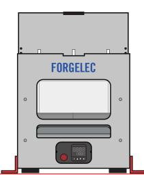
INSTALL FORGE **on Level Surface**With the Corner Plates
